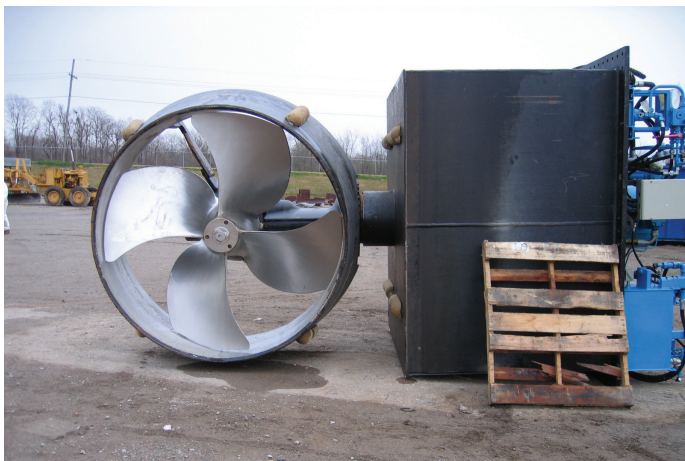
Z-drive propulsion/control unit.
