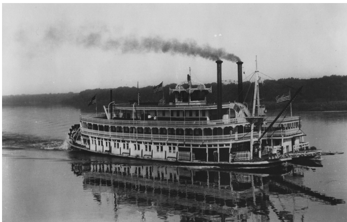
W.W. was former CITY OF WINONA , rebuilt in 1905 and renamed in honor of Capt. D. Walter Wisherd, friend of John Streckfus. Remained in Streckfus Line until 1917. Carried a barge alongside for additional excursionists. 137x29x4. Engines 13's with 5 ft. stroke.
