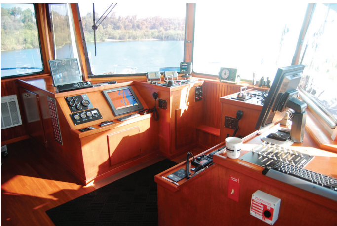
Pilothouse of Southern Towing Company's new Z-drive towboats. Note all the modern devices - no wheel, no sticks.
