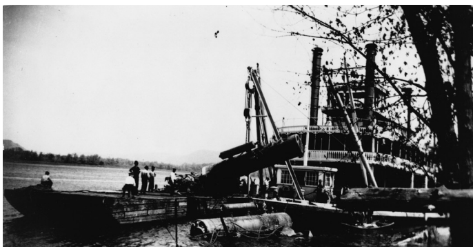
Government snagboat DAVID TIPTON raising boilers from the wreck of the J.S. at Bad Axe Bend after she burned, a total loss on June 25, 1910. Of the 1100 aboard, there were two casualties.
