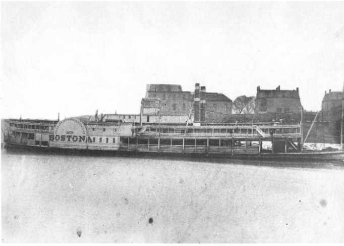
BOSTONA (0693) built 1879 at Cincinnati for Cincinnati, Portsmouth, Big Sandy & Pomeroy Packet Co. 302.5x43.5x6.7 engines 25's with 8-foot stroke having Frisbie valve gear. Dismantled 1899, machinery going to INDIANA.
