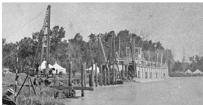
BIG HORN (0617) built 1865 in New Albany, 154x33.5x4.5. Engines 16's-4 foot stroke. Ran on Missouri River until fall of 1869, then on Red and Lower Mississippi. Sank and lost at Bayou Bartholomew, LA April 10, 1873.
