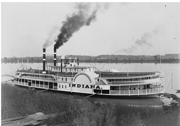
INDIANA (2754) built 1900 by Howard for L&C Packet Co. Hull was 285x45x6 with machinery from BOSTONA. Partially burned in 1916 and subsequently rebuilt by Howard into AMERICA shown below.
