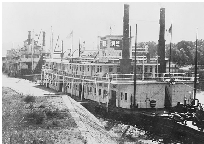
WAKEROBIN (5680) built 1926 by Dravo for U. S. Lighthouse Service. 182x43x5.3 Frisbie engines 18's with 7 1/2-foot stroke. Sold 1955 to Comet River Co., Cincinnati, for landing boat. Later acquired by Capt. Dennis Trone.
