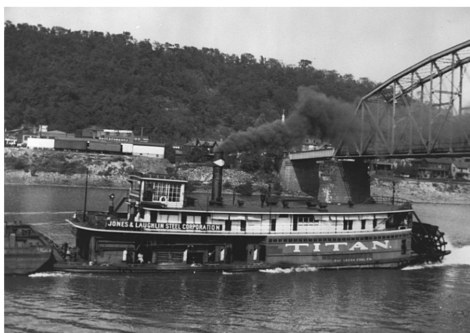
TITAN (T2443) built 1930 by Howard for Jones & Laughlin Steel with sister boat WM. LARIMER JONES. 136x34x7.3 with condensing engines 14's and 28's, 8-foot stroke. Among first boats to be steered by levers. Sold for scrap in 1953.
