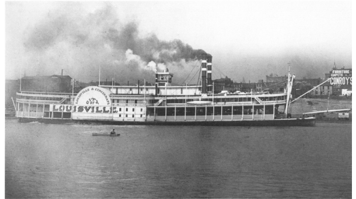
CITY OF LOUISVILLE (1095) built 1894 by Howard for L&C Packet Co. 301x42.7x7 with Frisbie engines 30's with 10-foot stroke. Ran Louisville to Cincinnati on April 18, 1894 in 9 hours 42 minutes, her time never beaten. Made record downstream run on April 5, 1896 in 5 hours 58 minutes. Lost in ice with CITY OF CINCINNATI on January 30, 1918.
