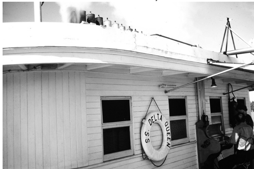
A set of Nichol/Van Splunter whistles on Quinby's straight-shot manifold: the design for the DELTA QUEEN calliope in this 1961 snapshot. Harmon Mize at the Shepard Labs keyboard. Photo courtesy Mike McDonald, Leavenworth, KS.
