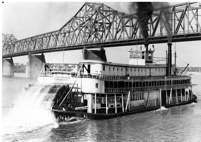
TOM GREENE (5415) built 1923 by Marietta Manufacturing for Greene Line Steamers. 200x38x6 with Frisbie engines 22's, 7-foot stroke. Won two celebrated races with BETSY ANN in 1929 and 30. Sold 1950 to Commercial Barge Line.
