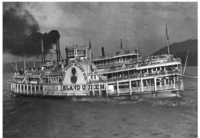
ISLAND QUEEN (2799) built 1896 by Cincinnati Marine Railway for Coney Island Co. 281.4x42.6x8.5 Engines 20's and 35's with 9-foot stroke. Burned at Cincinnati Nov. 4, 1922 with MORNING STAR, TACOMA, and CHRIS GREENE.
