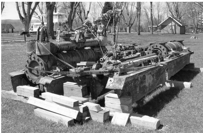
Present day photo of WAKEROBIN condensing high-pressure engines, 18's with 7½-foot stroke.
