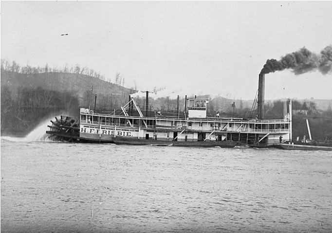
H. F. FRISBIE (T1010) built 1885 at Cincinnati for Huntington & St. Louis Towboat Co. 169.4x32.2x5.8 Engines 20's with 8-foot stroke. Dismantled 1903, machinery going to SARAH EDENBORN, later RENOWN, BOL wharfboat.
