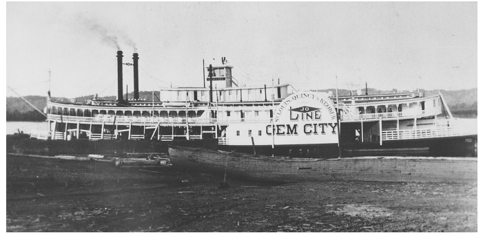
GEM CITY No. 2 (2222) was also built at St. Louis in 1884 with hull 263 x 29.8 x 5.6. Engines 20's with 7-ft. stroke. Her cabin and machinery came from ALEX MITCHELL. Ran St. Louis - Keokuk. She was bought in 1891 by Diamond Jo Line (as pictured above) and rebuilt into QUINCY at Dubuque's Eagle Point Boatyard in 1895. Acquired in 1911 with remainder of Diamond Jo fleet by Streckfus Steamers, and rebuilt into their flagship, J. S. DeLUXE in 1919. Dismantled 1938-39.
