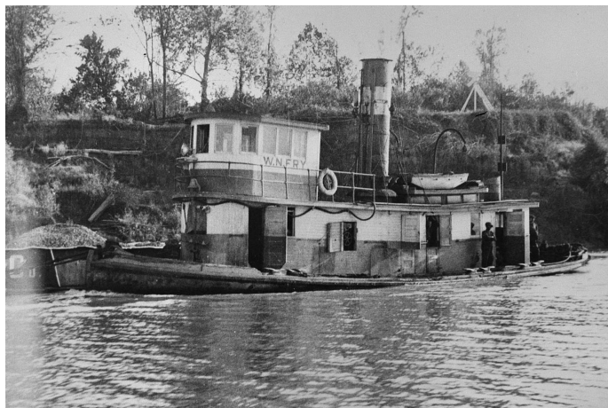
Propeller tug W. N. FRY, originally built as J. B. O'BRIEN at Pittsburgh in 1878 with hull 70 x 16 x 7. Ran as S. S. PRENTISS from 1900-25 until sold to Greenville Gravel Co.
