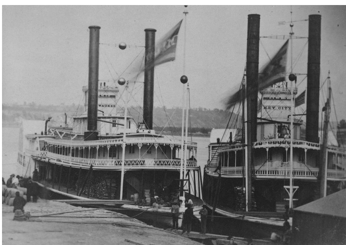
MILWAUKEE No. 2 (3936) and KEY CITY No. 1 (3278) pictured around 1862. KEY CITY , named for the city of Dubuque, was built at Cincinnati 1857, with hull 230 x 35 x 5.6 Engines were 20's with 7-ft. stroke. She sank the BEN COURSIN in collision near La Crosse in August 1857. MILWAUKEE was also built in Cincinnati that year, slightly larger by 43 tons. Ran Prairie du Chien - St. Paul. Both boats dismantled at Madison, IN in 1869.
