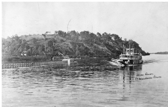
FLORA (2062), sternwheel packet built at California, PA in 1855 for Capt. Samuel Dean of Pittsburgh, before heading to Upper Mississippi for William Davidson. 152 x 19.3 x 3.9, 160 tons. Shown here passing Ft. Madison, IA. One of the low water boats mentioned in this article.
