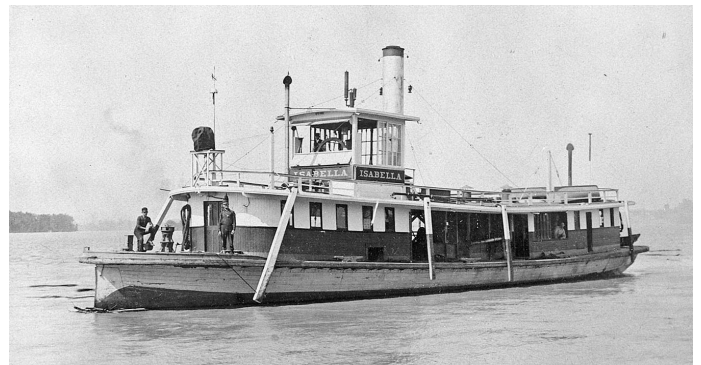
ISABELLA (T1213) built 1880 at Evansville, IN. Capt. Way says she was a wood hull prop tug 95.5 x 22 x 4.8, and towed transfer barges for the L&N Railroad. All photos on pp. 14-17, except as noted, are courtesy of Murphy Library, University of Wisconsin, La Crosse
