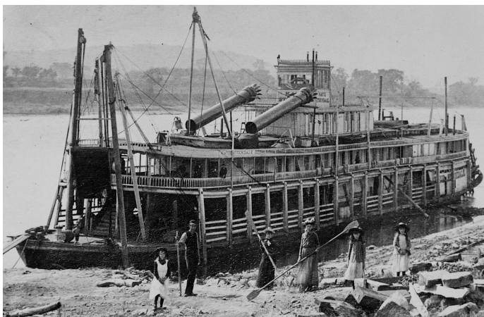
KATIE STOCKDALE (3253) , 228 x 34.5 x 5 hull built 1877 at California, PA and completed at Pittsburgh. On Feb. 10, 1884 her pilohouse was sawed off level with pilotwheel to allow her to pass under Parkersburg bridge.
