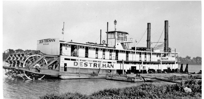
DESTREHAN (T0594), 133.9 x 32 x 5.4. Built by Ward Engineering, Charleston, for Pan American Petroleum Co. She towed gasoline from New Orleans to Pittsburgh spring 1934, and Wood River-New Orleans in 1937. Photo from Murphy Library, University of Wisconsin-LaCrosse.
