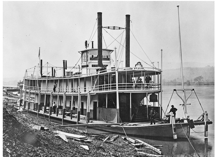
COLBERT (To461) built 1891 in Jeffersonville for U. S. Engineers with engines 10 3/4 by 4 1/2 foot stroke. Steel hull placed by Nashville Bridge in 1925 measuring 137.9 x 26.2 x 4.5. Capt. Paul Underwood was Master in her later days. Photo from Murphy Library, U W - La Crosse
