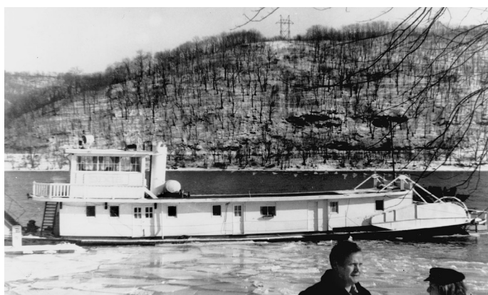
DIXIE , 76.5 x 18.8 x 4, built in 1937. Probably the last diesel sternwheeler built by NABRICO. Murphy Library photo.
