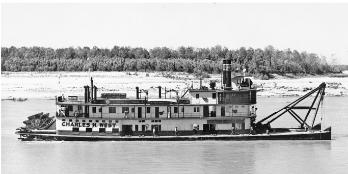
CHARLES H. WEST (T0381), 195 x 38 x 7.6 towboat/snagboat built 1934 for Vicksburg U. S. Engineers. Iowa Machine Works compound engines 14's and 28's with 6-foot stroke. Decommissioned in 1958 and rebuilt as floating restaurant LT. ROBERT E. LEE at St. Louis. Burned in March 2010. Photo from Murphy Library, U W - La Crosse.
