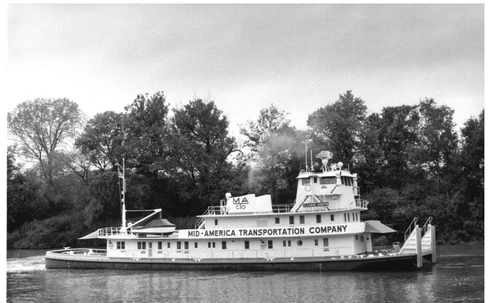
ELEANOR GORDON shown in official NABRICO portrait. Built for Mid-America Transportation Co. in 1956, twin prop 149 x 35. A classic example displaying the lines of a Nashville-built boat. Photo courtesy of Boat Photo Museum.
