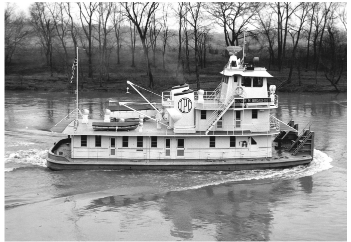
NELSON M. BROADFOOT at Nashville. Built 1949, twin prop 80 x 30 x 10 for Ingram Barge Co. and named for Capt. Nelson M. Broadfoot (1893-1953), vice-president and director of Ingram at the time. Photo by Boat Photo Museum.
