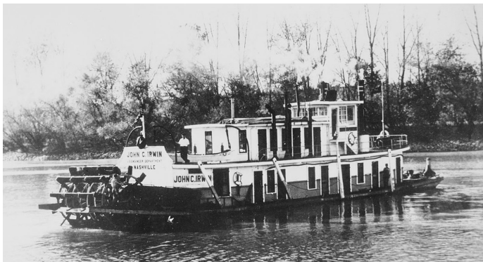
JOHN C. IRWIN at Nashville on October 25, 1935. Built in 1924 for U. S. Engineers with hull 98 x 20 x 4.5 Murphy photo
