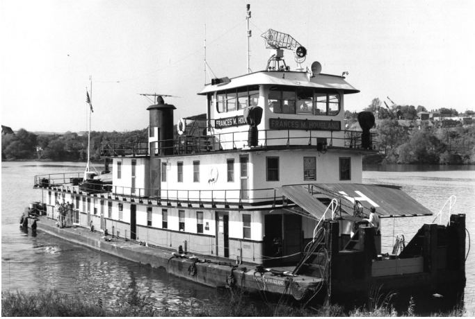
FRANCES M. HOUGLAND on Oct. 4, 1963 at Monaca, PA, pushing into water plant to take on drinking water. Built 1947 for Houglan Barge Line, twin prop, 128.5 x 28 x 8.5. Photo courtesy of Boat Photo Museum.
