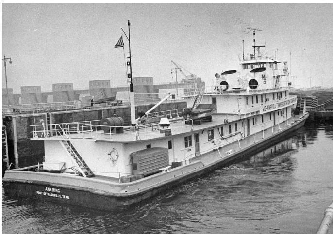
ANN KING upbound in Upper Mississippi River lock. Built for Mid-America Transportation Co. in 1964. Twin prop with Kort nozzles, 165 x 35 x 10.4. Photo from Murphy Library, University of Wisconsin - La Crosse.
