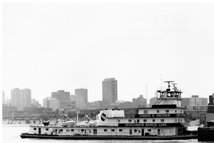
JAMES E. SNYDER upbound at St. Louis on May 27, 1977. Built 1976 for Wisconsin Barge Line of Cassville, WI. Triple prop, 195 x 54. Sister boat to JIM BERNHARDT and MISS KAE-D. This trio, along with HARRIET ANN of 1966, are the largest built by NABRICO. Photo by Boat Photo Museum.
