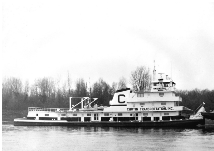
OLINDA CHOTIN shown at Brookport, IL above Lock and Dam 52 on the Ohio River on November 22, 1967. Built that year for Chotin Transportation, Inc. of New Orleans. Twin prop, Kort nozzles, 154 x 48. Photo from Boat Photo Museum.
