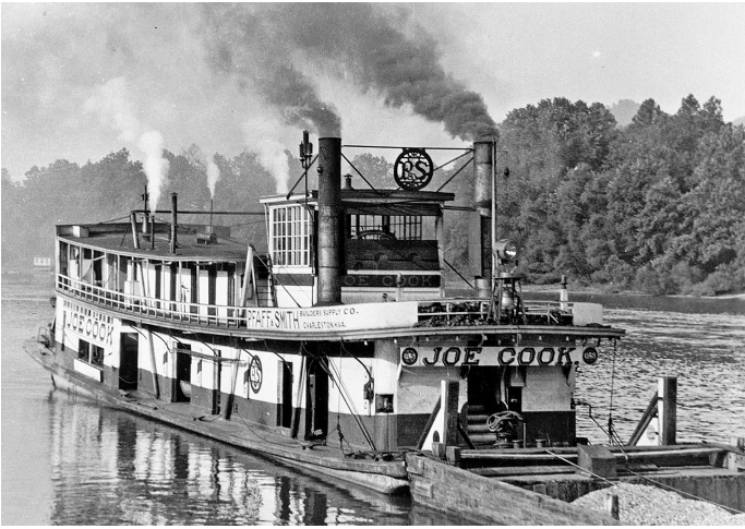
The hull of JOE COOK (T1384) built 1930 by NABRICO. Engines were 12's-5 from towboat WESTERN, replaced in 1947 with 16's-5 from snagboat KENTUCKY. Exploded a boiler at Ravenswood, WV Apr. 1, 1947, claiming 3 lives. Last boat to blow QUEEN CITY whistle. Murphy Library photo.
