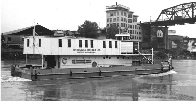
CATERPILLAR , twin prop 100 x 25 x 8, built 1949 for NABRICO. Used as party boat, as she had a large galley, and helped deliver new barges and towboats to Paducah. The venetian blinds below pilothouse shielded an open-air veranda where guests of the new boat could view the river. NABRICO erection yard is behind boat with company offices behind pilothouse. Photo courtesy of Boat Photo Museum.
