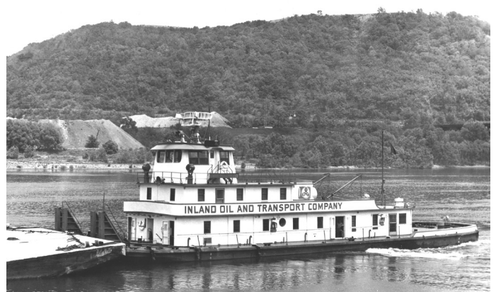
LADY ROSE-MARY shown May 29, 1964 upbound entering old Lock 10 at Steubenville, OH. Slag pile from Weirton Steel Company in left background. Built 1957 for Inland Oil and Transport Co., twin prop 130 x 30 x 10.5 Photo courtesy of Boat Photo Museum.
