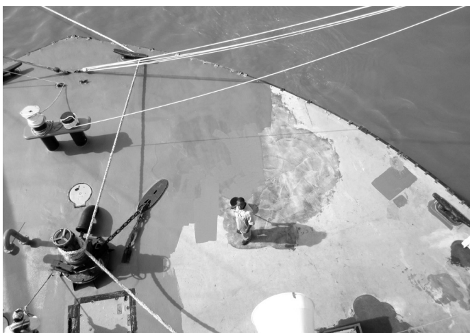
New traditional steamboat red deck enamel going on the bow.
