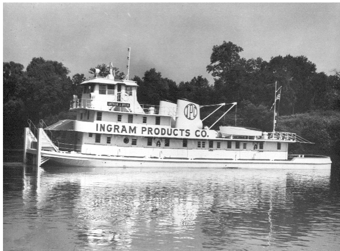
m/v ARTHUR J. DYER, 124 x 27.5 x 11.3, twin prop, pictured when new. Built in 1951 for Ingram Barge Co. Photo courtesy of Public Library of Cincinnati and Hamilton County.
