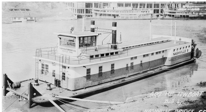
NASHVILLE B. when new at NABRICO yard in 1926. Hull 111 x 29.4 x 5.6 From Murphy Library, U W - La Crosse.
