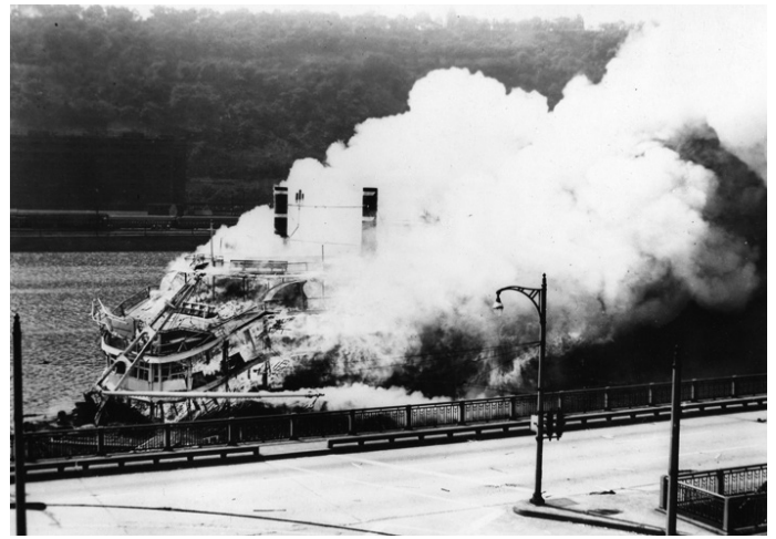
Forward end of ISLAND QUEEN collapses after fumes in fuel bunkers ignite and explode Sept. 9, 1947. Capt. Wagner was likely in the water by this time after helping others escape. Public Library of Cincinnati and Hamilton County photo.
