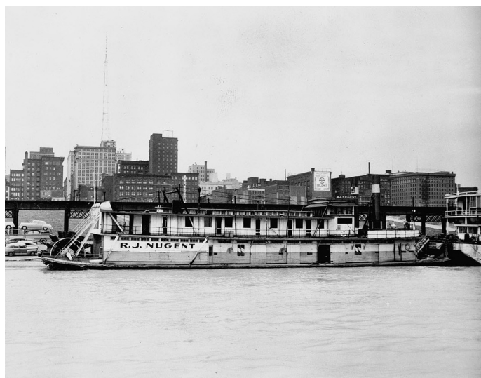
R. J. NUGENT (T2093) built in 1912 at Cincinnati as U.S. Engineer towboat SCIOTO. 157 x 31 x 4.2, with engines 14's - 6 foot stroke. Capt. Harry Loudon, DELTA QUEEN Ohio River pilot of the 60s, 70s and 80s, served on this boat during his career with the Corps. Renamed by Nugent Sand Co. of Louisville when they bought her in March 1948. At the end of that same month, she collided with the GORDON at Twelve Mile Island, resulting in damage to both boats. Capt. Cuba A. Foster of the NUGENT suffered minor injuries. Sold in April 1951 to J. W. Menke of St. Louis, and then to Bernard Bros. Auto Supply of New Iberia, LA in 1953 for use as a quarterboat. Photo from Murphy Library, U W - La Crosse.
