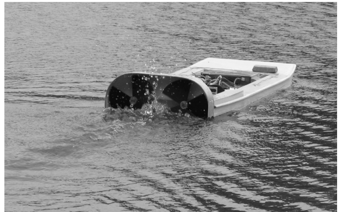
Test run: underway on vane wheel power! As you can see, they throw water all over.
