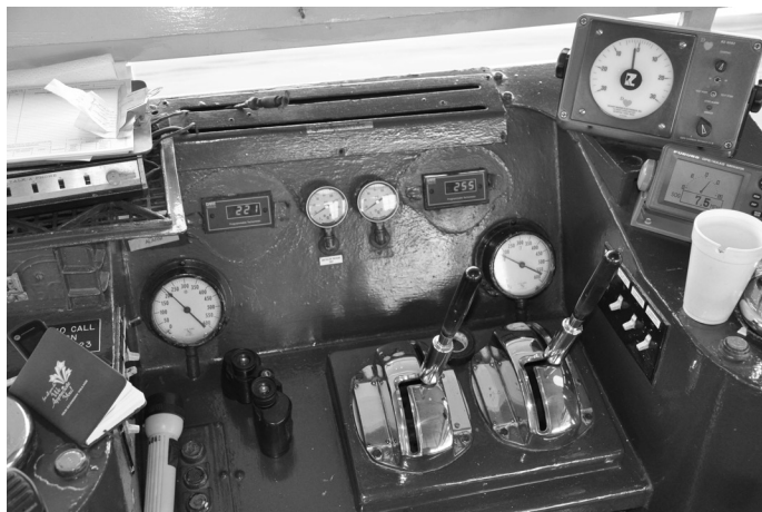
Pilothouse console, complete with brass engine controls.
