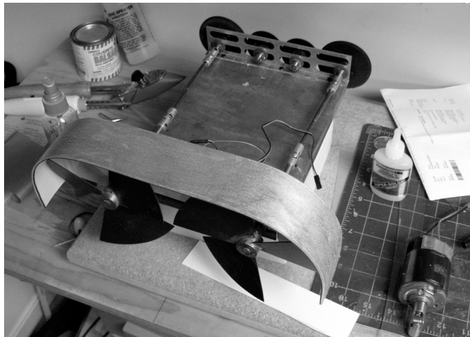
Vane wheel drive unit, built on sheet brass base and attached to hull with three screws. 12V electric motor sits on bench.
