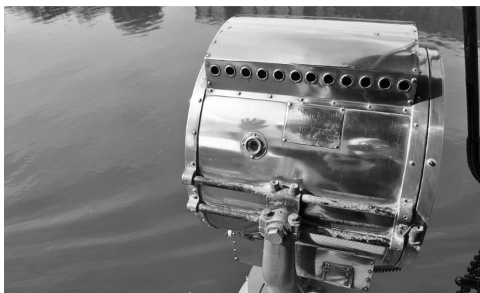
Pilot Mark Handley on watch in glass-enclosed pilothouse, amidst the gleam of highly polished brass fixtures. Below, the vintage Carlisle and Finch carbon arc searchlight.
