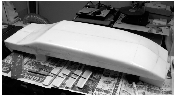
37" model towboat hull on workbench. Note the four rudders lying in front. Only three were used and have worked out well.
