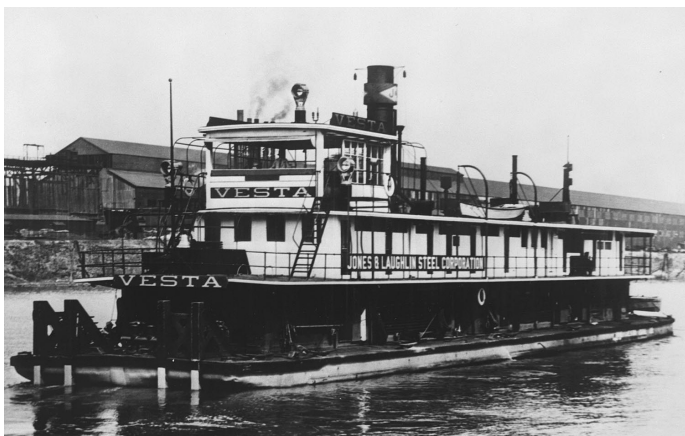
J&L's new towboat VESTA. Originally powered by triple expansion condensing engines 10's, 17's, 21¼ with 18-inch stroke, rated 750 hp. Photo from Murphy Library, La Crosse.
