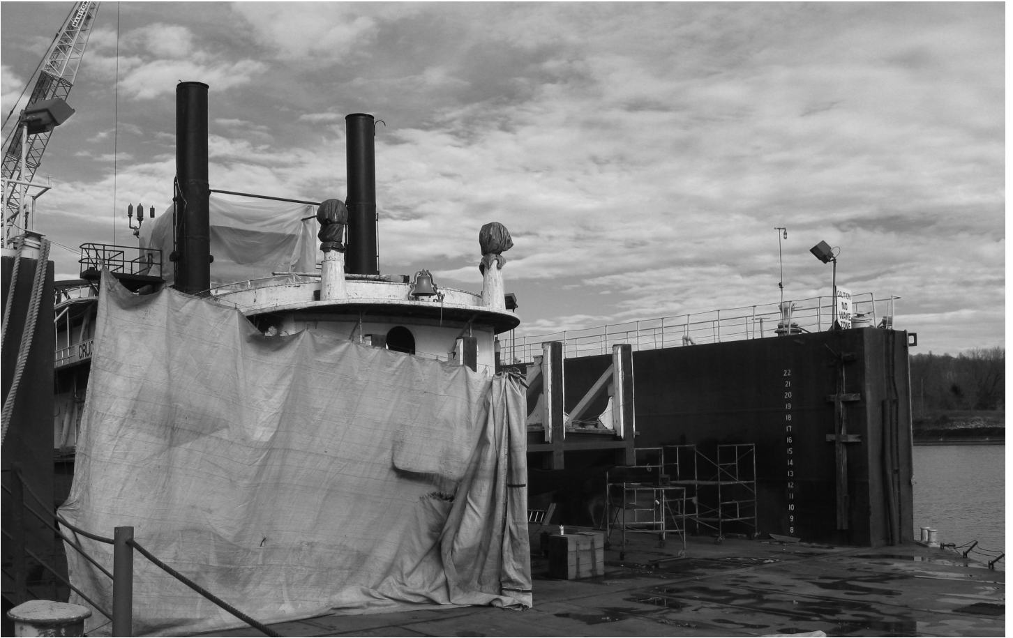
SNYDER on drydock with tarp providing some protection for work crews during chilly November days. Shipyard crews at work during winter months labor in typically inhospitable conditions on the Ohio, Kanawha and Upper Mississippi Rivers.
