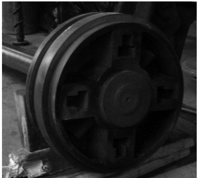
Starboard piston with endplate and bolts removed. This is probably original with the boat. Both photos by Dan Lewis.
