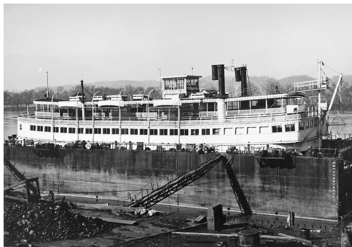
On drydock at Marietta Manufacturing Co. in Point Pleasant, WV, spring 1955 for addition of sponsons to her hull. Both photos from editor's collection.
