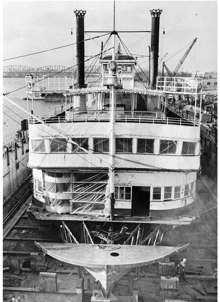
Alan Bates designed a new bow for the boat and faired her boxy sponsors into the existing hull. Photo from Murphy Library.
