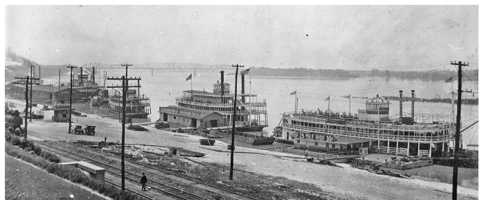
Top: IDLEWILD after her texas roof has been carried all the way to the after end of the skylights. The Safety First signs on her pilothouse remained until the tiller lines were re-routed through the front sides of the pilothouse. Center: Sign on WMPCo. wharfboat advertises all-day round trip for 75¢ and 25 mile trip for 50¢. Bottom: Lee Line's PRINCESS on far right has undercut IDLEWILD's 25-mile round trip fare by 15¢. Top photo from editor's collection; center and bottom photos from Murphy Library, Univ. of Wisconsin - LaCrosse.
