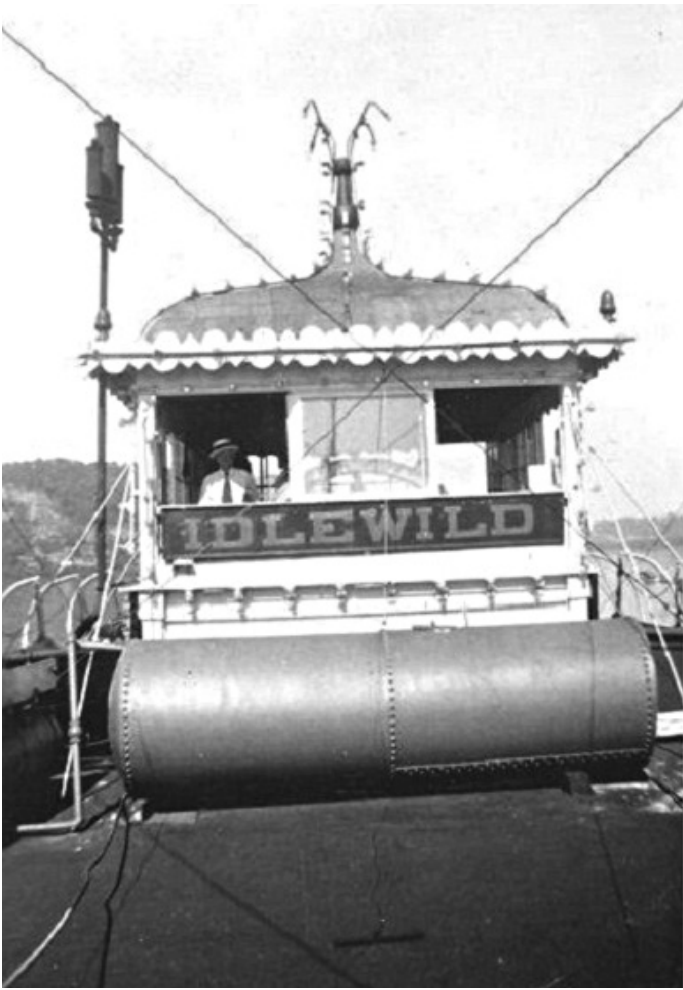
This view of the front of the pilothouse shows the water tank on the roof with an old-fashioned tank type life float to the left. The pilothouse lights on the dome and on the Christmas tree display atop the dome clearly show in this view.
