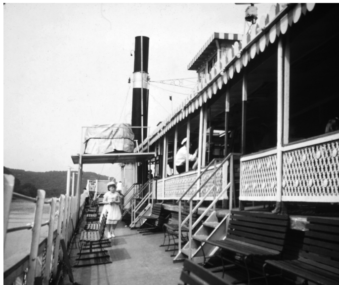
Above: Hurricane roof and texas looking forward on port side in 1957. Below: Three years later, the old wire mesh railing around the edge of the hurricane roof had been replaced with sturdier steel bulwarks in this same location looking aft.
