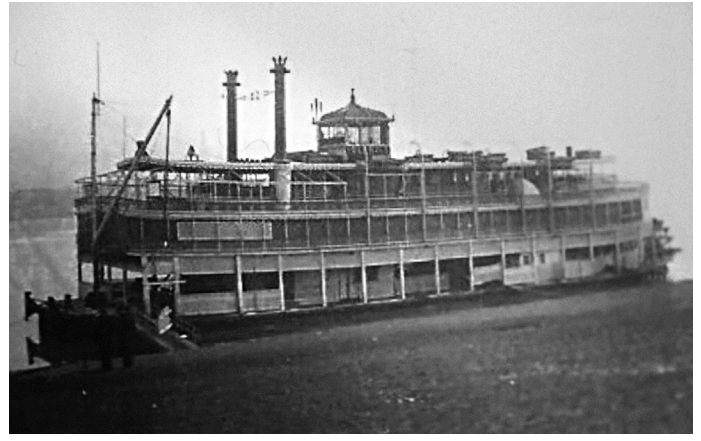
Rare photo of the boat taken during her World War II service for the government showing the tow knees that were riveted to her bow. They had also been fitted earlier when she towed on the Missouri in the late twenties. Murphy Library photo.
