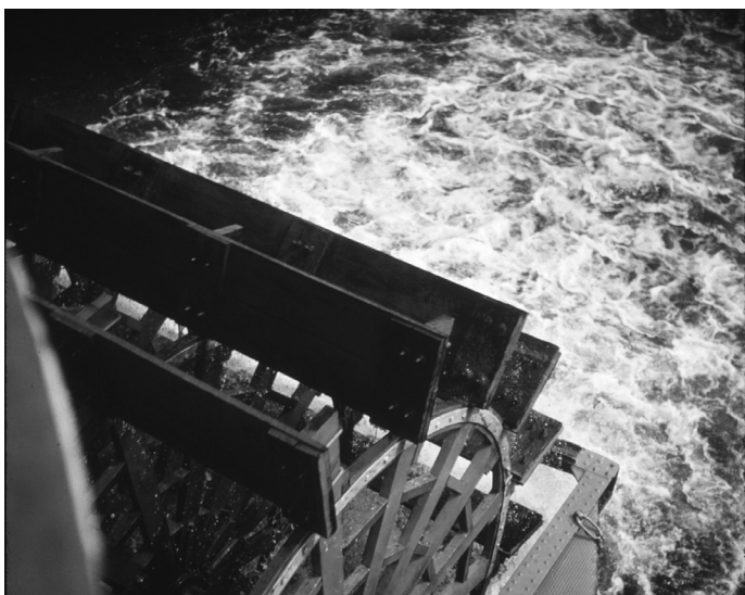
Sternwheel was built of white oak, 24 feet long by 19 feet in diameter, with 16 buckets having a two-foot dip and an ad.
