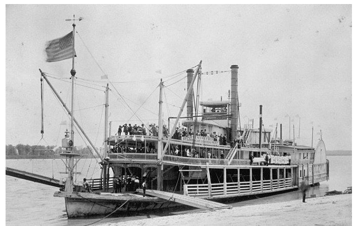
Samuel Stacker Lee was captain on IDLEWILD (2726) beginning in 1876. Built in 1870 by Howards for the Cairo-Paducah-Evansville trade, she was eventually sold to Memphis & Arkansas City Packet Co. Measuring 216 x 35.6 x 6.4, her engines were 22's with 6½-foot stroke. She burned at Memphis July 31, 1881. Murphy Library photo.
