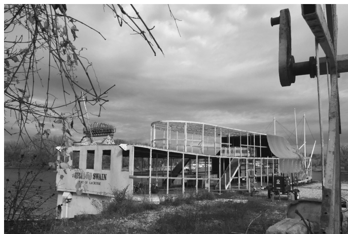
Cabin deck looking forward. A hydraulic lift for passengers will be installed to provide access to the main deck.
