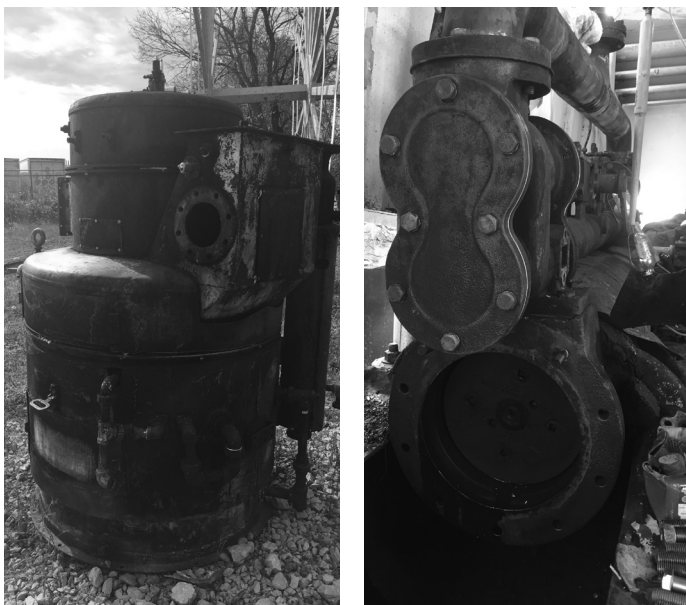
Left: Old boiler removed from hold sits on shore. Right: With cylinder head removed from starboard engine, piston head is readily visible. These are patented Gillett & Eaton slide valve engines 12's-5 ft. built for CITY OF BATON ROUGE.
