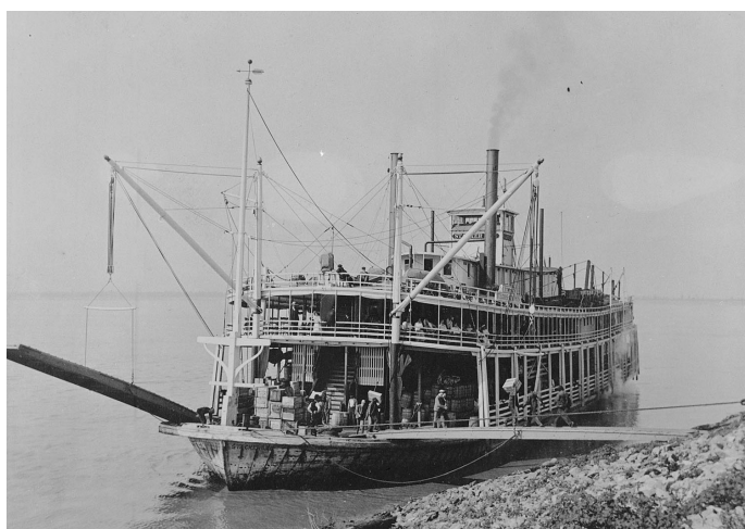
STACKER LEE (5174) came out in 1902 with engines 18's-8 ft. stroke powered by three boilers on a hull 225.5 x 45 x 6.5. Ran St. Louis-Memphis. Courtney Ellis, a Lee Line engineer, recalled a sign over the crew's table which warned "No Steamboating at Meals." Murphy Library photo.
