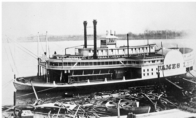
The second JAMES LEE (2934) when brand new at Howard Shipyard in 1898. Built for $27,000, she carried engines 24's-8 ft. stroke on a hull 230 x 43 x 7. She ran Memphis-Friar's Point with Capt. John Darragh. Capt. Way comments: "This was a handsome boat, consistently successful, and outlived her usefulness as a packet." She was converted into an excursion boat in 1917 and renamed DE SOTO. Murphy Library photo.
