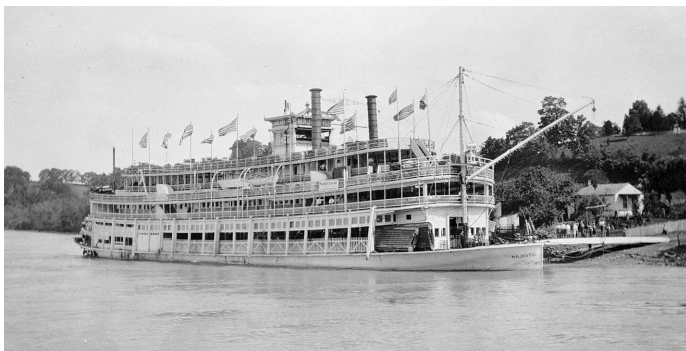
Second MAJESTIC (3712) was originally S.S. BROWN, then REES LEE. Capt. Wisherd's partner in converting this 228 x 44 x 6.6 Ambridge, PA-built steel hull steamer was Capt. Peters Lee. Complete story of BROWN-LEE-MAJESTIC appears in June 1972 REFLECTOR. Photo from Murphy Library.
