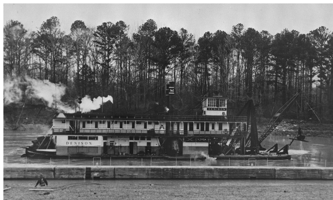
DENISON, steam snagboat built 1915 by Dubuque Boat & Boiler Co. for USE at Mobile, AL on Warrior-Tombigbee Rivers. G&E engines 12's - 5 ft, 250 hp. Murphy Library photo.
