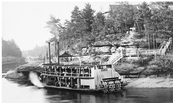
Wisconsin Dells excursion steamer APOLLO was built at the Dells in 1898 with G&E engines 8 inches by 3'-8" stroke. A new APOLLO II was built in 1971. Murphy Library photo.
