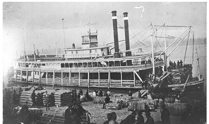
Although the sinking of JAMES D. PARKER (2920) at the head of the chute on March 5, 1882 was the most serious accident Capt. Pink encountered in his long career at the Falls, no injuries resulted. The 185 x 36 x 5.5-foot PARKER was built in 1872 at Cincinnati for the Memphis & Ohio River Packet Company. Photo courtesy of Murphy Library, University of Wisconsin-LaCrosse.
