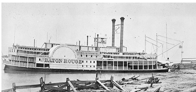
CITY OF BATON ROUGE (1050) above and CITY OF NEW ORLEANS (1112) below were both Howard-built in 1881. BATON ROUGE was slightly larger at 294 x 49 x 9’5”. Both were owned by Anchor Line for St. Louis-New Orleans trade. Their delivery below the Falls was entrusted to Capt. Pink. Both photos courtesy Murphy Library, UW-LaCrosse.
