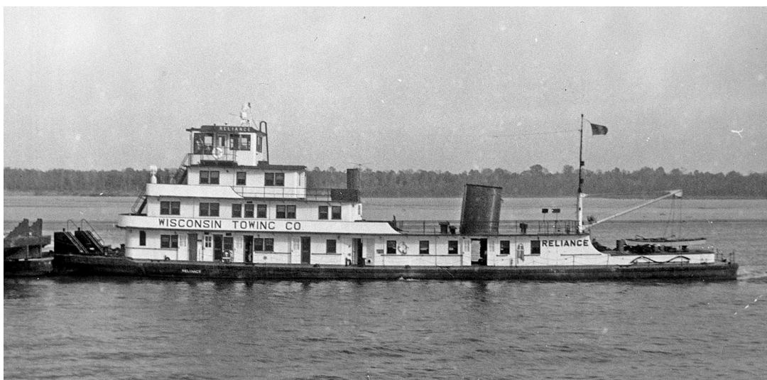
m/v RELIANCE built 1947 by Dravo Corp., Neville Island, PA. 167 x 36.5, twin screw. GM 16-567 AD diesels, repowered in 1966, 2000 hp. Photo from Murphy Library, UW - La Crosse.
