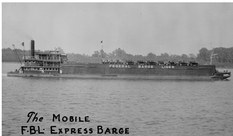
Above: Str. JAMES W. GOOD (T1340) with auto barge for delivery below St. Louis from Ford's Twin Cities Assembly Plant. Below: FBL "express Barge" MOBILE (T1844), 280.1 x 49.1 x 10 was a self-propelled freight barge, shown here carrying Fords in 1932. Murphy Library photos.
