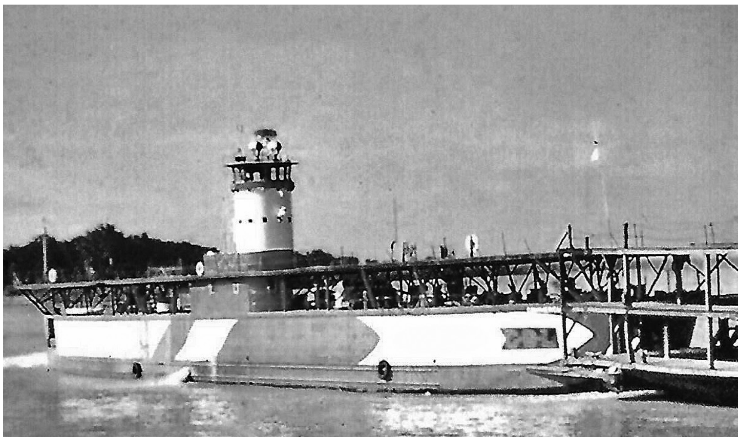
Before and After: Shown at top is LSM 220 (Landing Ship Medium), purchased by CBL as war surplus for conversion below into Car Carrier m/v COMMERCIAL DISPATCH. Work was done by St. Louis Ship in 1949. Photos by Capt. Bill Judd.
