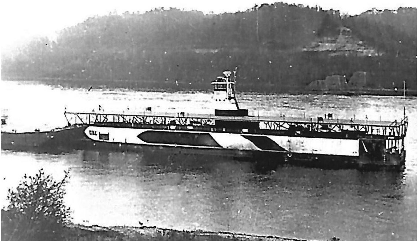
Top: Commercial Barge Lines super barge, one of four built by St. Louis Ship. Each barge had three levels of auto storage. Capacity was 240-280 cars each. They measured 560 x 35. This July 26, 1949 photo shows the barge in tow of COMMERCIAL TENNESSEAN at Cape Girardeau, MO. 137 new Fords are being delivered to St. Louis. Bottom: m/v COMMERCIAL COURIER, converted from LSM221 by St. Louis Ship in 1950. Pictured here waiting to load barges at the Cincinnati terminal in 1954. Top, next page: COMMERCIAL COURIER fully loaded with all three units. Middle, next page: m/v COMMERCIAL DIXIE waiting on autos to load at CBL dock in Louisville, 1950. Bottom, next page: m/v COMMERCIAL DIXIE, ex-mine sweeper AM235 FIXITY. Photo taken in 1949 after conversion to towing vessel at Paducah Marine Ways. Capt. Bill Judd photos.
