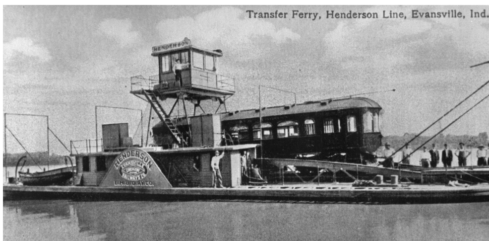
Left: Ferry HENDERSON with interurban car making the passage between Evansville, IN and Henderson, KY. Right: The street railway car about to roll onto the floating cradle. Note the huge pile of drift on the left. Both photos from Murphy Library.
